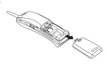
2. Slide the Battery Pack down into the Handset.
